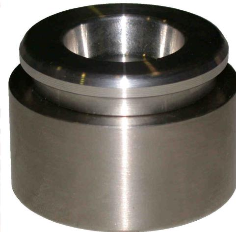
Fit the seals ([ref. 11](#)) on their respective pistons, in the same direction as the standard assembly, as shown in the photo opposite.
