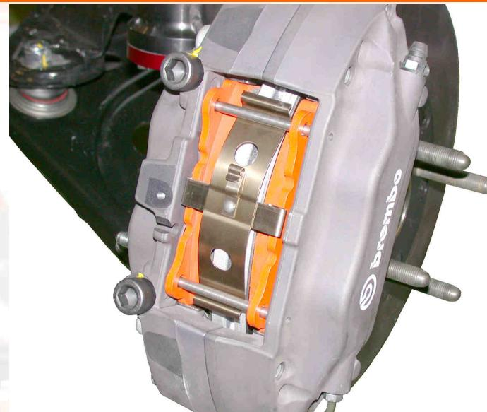
Connect the two brake pad retaining pins by lockwire, as shown in the photo opposite.
