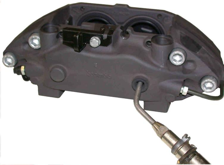
Remove the "bakelite" inserts, taking great care not to damage or scratch the pistons (reused).
